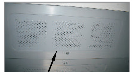
PA system speaker have been installed in the coach
